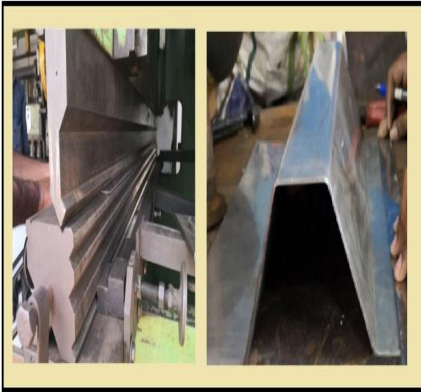
Figure 4: Fabrication Technique of Corrugated Core
